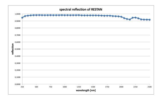
For comparison the PTFE reference included with the calibration board exhibits the below reflectance spectrum. We have included the reflectance spectrum of the PTFE reference and the corresponding wavelength axis in the files "PTFE\_Reference\_Reflectance.txt" and "PTFE\_Reference\_Wavelength.txt". This can be used to correct the datacube after intensity calibration if a higher precision reflectance cube is needed.
