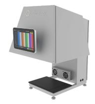
The Lab Scanner is a high-performance, all-in-one system for research and proof-of-concept development. It offers fast, high-resolution hyperspectral imaging with intuitive controls and offline spectral analysis. Featuring broadband halogen illumination, 300 mm scan width, and precise optics, it captures fine spectral and spatial details. Available with the Hypervision 1000 or 1700 cameras, it delivers flexible, accurate imaging for researchers and industry professionals alike.
